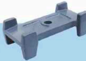
CODE NO. : SHBC 358 PART NAME : SPACER PLATE (BIGGER HOLE) VEHICLE : TATA 1612 / 1210 / SE PART NO. : 340 324 0335
